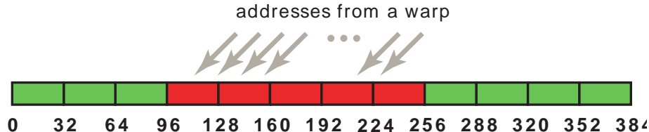
Figure 4 Misaligned sequential addresses that fall within five 32-byte segments
