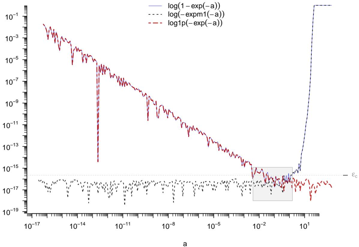
Figure 1: Absolute relative errors (with respect to 1024 bit **Rmpfr** computation) of the default,  $\log(1 - e^{-a})$ , and the two methods “**expm1**”  $\log(-\text{expm1}(-a))$  and “**log1p**”  $\log1p(-\exp(-a))$ . Figure 2 will be a zoom into the gray rectangular region where all three curves are close.
