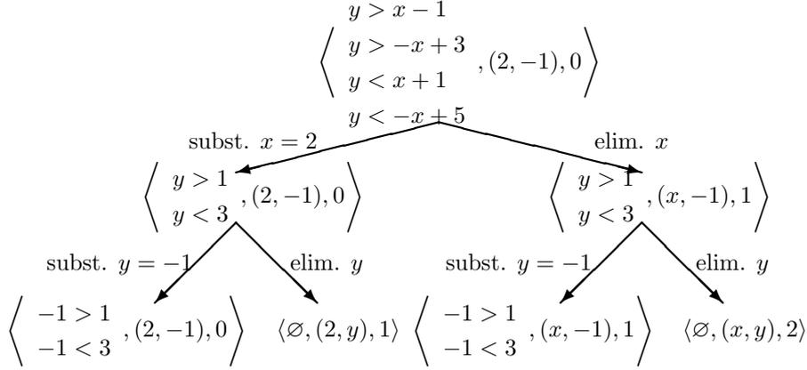
Figure 2. Graphical representation of the binary tree used to solve the error localization problem for the record  $(x = -2, y = -1)$ , subject to the edits of Eqn.(16). Each node contains an edit set, a (partially completed) record and the solution weight.
