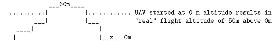
To avoid negative impacts from the Phantom 3 auto-calibration, the launch altitude is used to correct the flight altitude according to:
